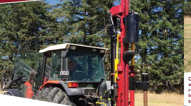
Optional spike with hydraulic retraction and hydraulic spike turner.
