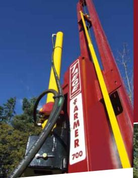
Strong proven twin box mast made of 6mm steel
