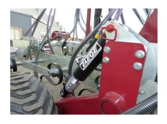
A simple but clever wing lock system is used so that when the wings are folded up the weighted lock system prevents the wing from folding in too far due to the slotted wing ram carriers.
