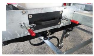
If higher rates are required a quick and simple cartridge change with fluted rollers fitted is all that is needed.
