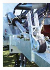
Strong, fully welded, hot dipped galvanised frame and brackets which insures longevity of your investment.
