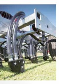
Very flexible '5' tynes set on a patented angle combined with Taege 3 piece boots and hard wearing narrow tungsten faced tips is a vastly different set up to other tyne drills.
